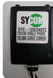
A Type 2 SPD is called a transient voltage surge suppressor (TVSS). A TVSS must be installed on the load side of the service entrance main and be 600 volts or less. Type 2 devices should be installed by a licensed electrician according to the manufacturer's guidelines.
